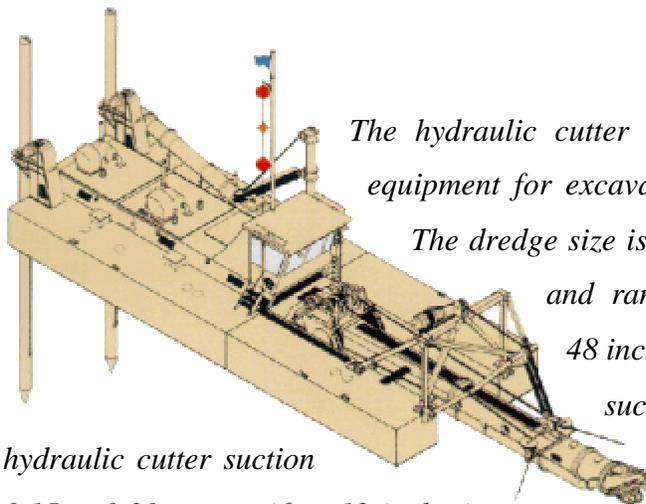
*The hydraulic cutter suction dredge is the most commonly used equipment for excavating and maintaining navigable waterways.*
